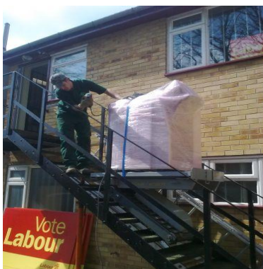
Figure-5: Lifting Load with Stair climbing Vehicle
