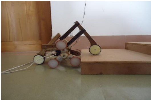
Figure-25: Vehicle climbing stair from flat ground
